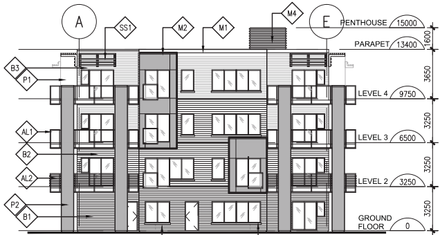
6 East Elevation - Building 2 A401 SCALE: 250
